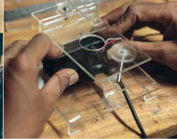
Workshops to build a computer-compatible microscope out of a webcam have already been carried out worldwide.
